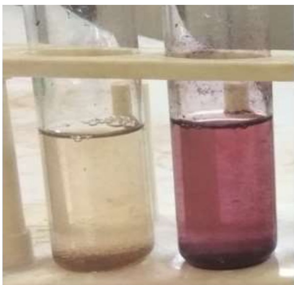
Figure 1. Colour change in the reaction mixture indicate formation of AuNPs.
